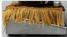
SY-2200 地毯须边机 Carpet fringing & over edging machine
